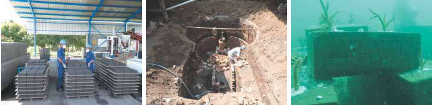
⚡ PT YTL Jawa Timur's FABA paving block production (left), used in one of the 680 biogas units (center) and reef blocks (right) near the power plant
