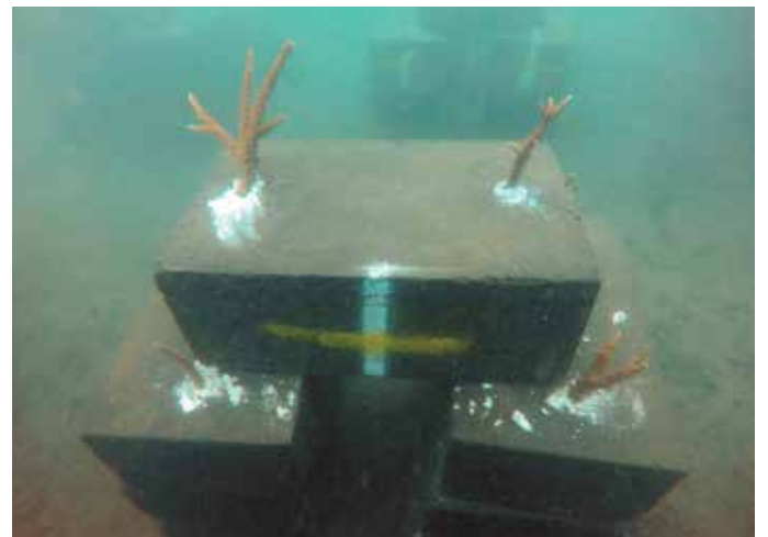
Coral seen here transplanted on blocks made from the coal-fired power plant waste - Fly Ash and Bottom Ash (FABA)
