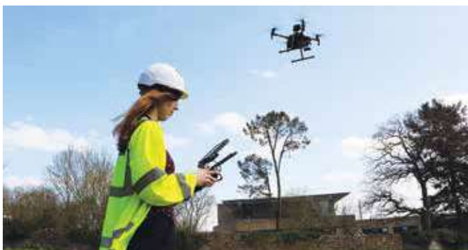
» Wessex Water deployed ten unmanned aerial vehicles, fitted with leak-spotting thermal imaging cameras, to help them in detecting leaking pipes during cold spells
