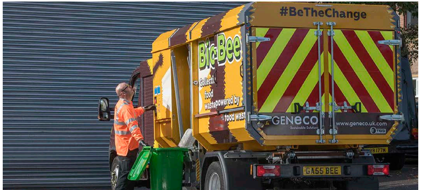
Food waste is collected in the Bio-Bee and brought back to GENeco UK’s anaerobic digestion plant in Bristol. The waste is depackaged - and plastic is removed - and is then used to produce sustainable biomethane derived electricity for homes and communities
