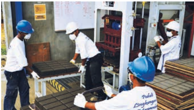
— Paving block production using fly ash and bottom ash as alternative raw materials
