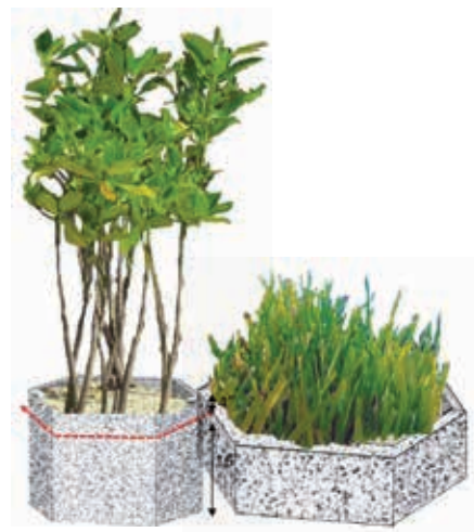
The hexagonal concrete box design for seagrass
