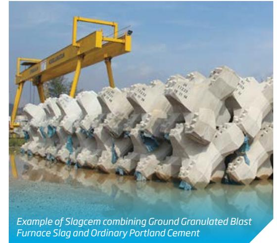
Example of Slagcem combining Ground Granulated Blast Furnace Slag and Ordinary Portland Cement
