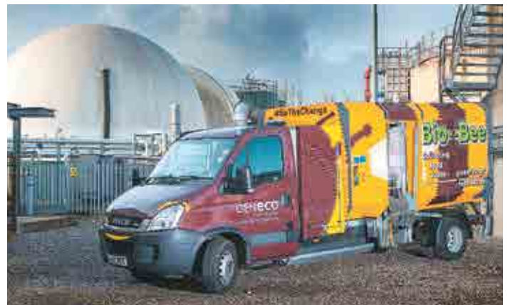
GENeco UK's Bio-Bee vehicles both collect commercial food waste and run on biomethane from the same waste
